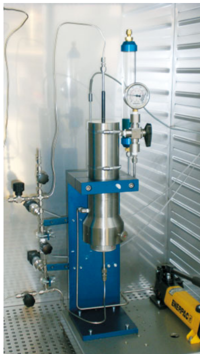
Fig. 3. Hassler type core holder
