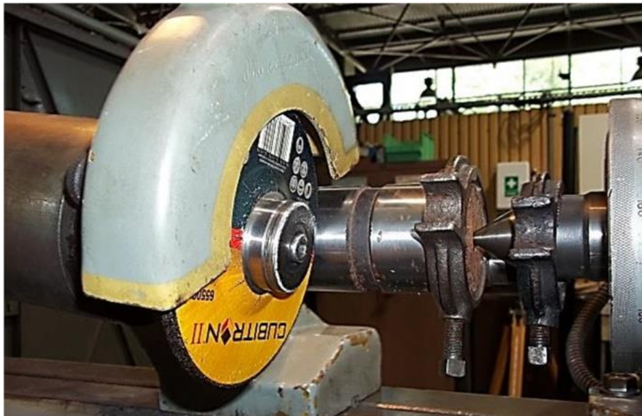
Fig. 13. Zone of grinding with a Cubitron™ II grinding wheel
