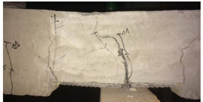
Fig. 7. Destruction of sample BD-3 due to rupture of the rebar
