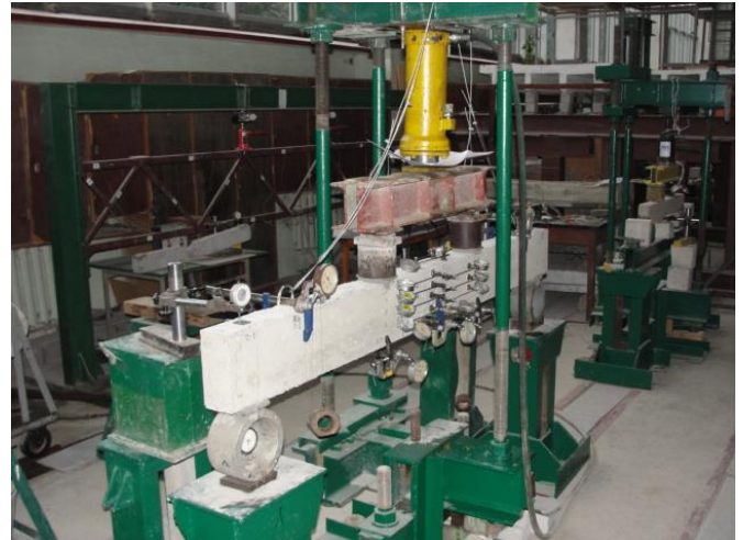
Fig. 3. General view of experimental stand and location of devices
