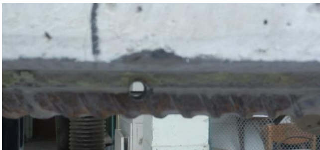
Fig. 2. General view of a single hole in the reinforcement of damaged samples BD-3 and BD-4
