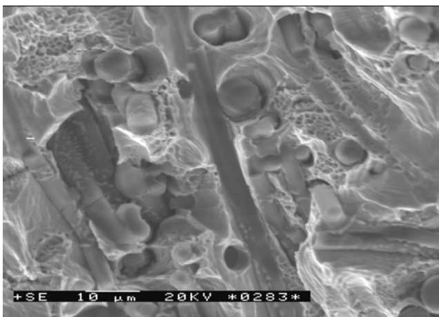
Fig.3. Fracture of Cu based composite materials reinforced with 10% of Al 2 O 3 fibres
