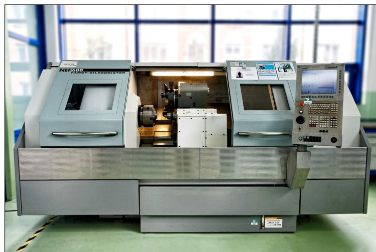
Figure 3. Test stand – NEF 600 lathe
