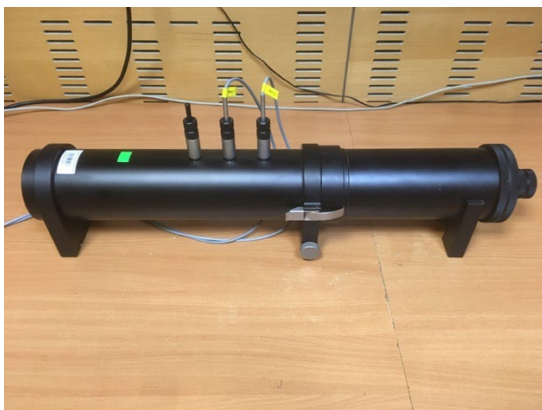
Figure 8. Impedance tube for measuring the sound absorption coefficient.
