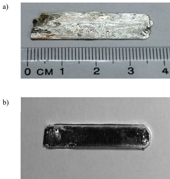
Fig. 1. Samples of Mg_{66}Zn_{30}Ca_4 in the form of plate with 2 mm (a) and plate with 1 mm (b)
