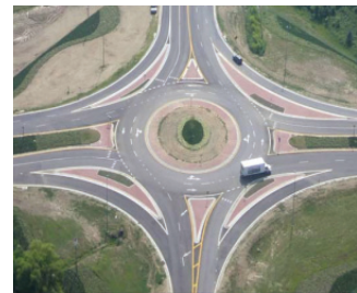
Fig. 3. Conventional Roundabouts with bypass lane
