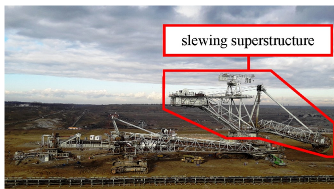
Fig. 1. BWE SRs 2000×32/5+VR92 on the surface mine 'Tamnava West Field' (Serbia): theoretical capacity 6600 m 3 /h, total mass 2905 t
