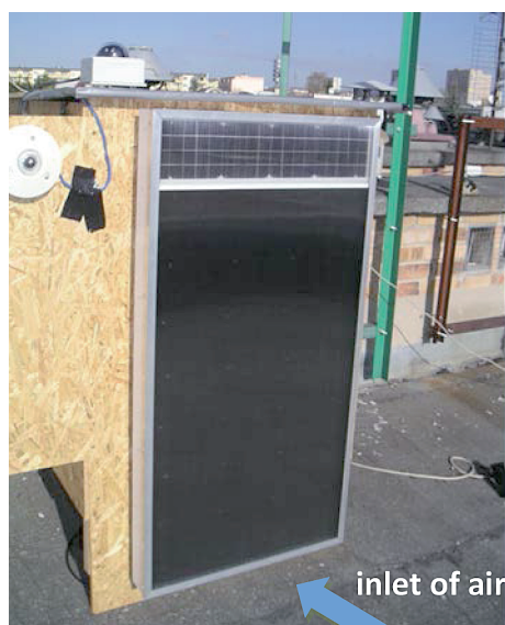
Fig. 1. Measurement station with the vertically installed solar air collector and sensors for measuring the radiation
