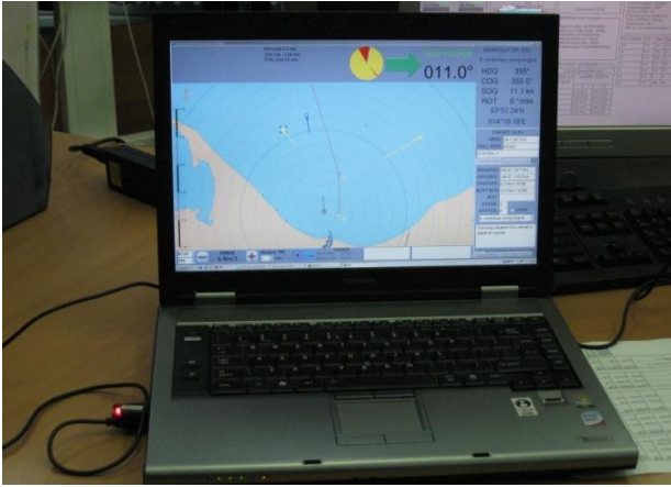
Fig. 1. NAVDEC, installed on the m/v “Navigator XXI”
