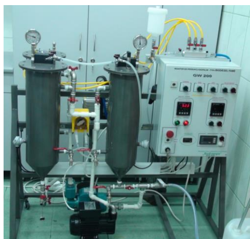
Fig. 2. Reactor GW 200 for production of Biodiesel FAME (SME)
