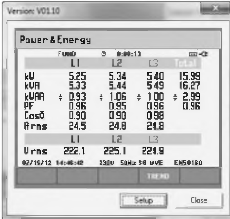
Fig. 6. Measurement results of active, reactive, and apparent power values (total values and in particular phases), the values of phase current and voltage and the power factors in case of the following devices connected to the mains: a) a three-phase capacitance receiver; b) the UPS operating at effective load equal to 100% P_m ; c) the UPS and capacitance receiver connected in parallel; d) the UPS and capacitance receiver connected in parallel with adjusted reactive power compensation
