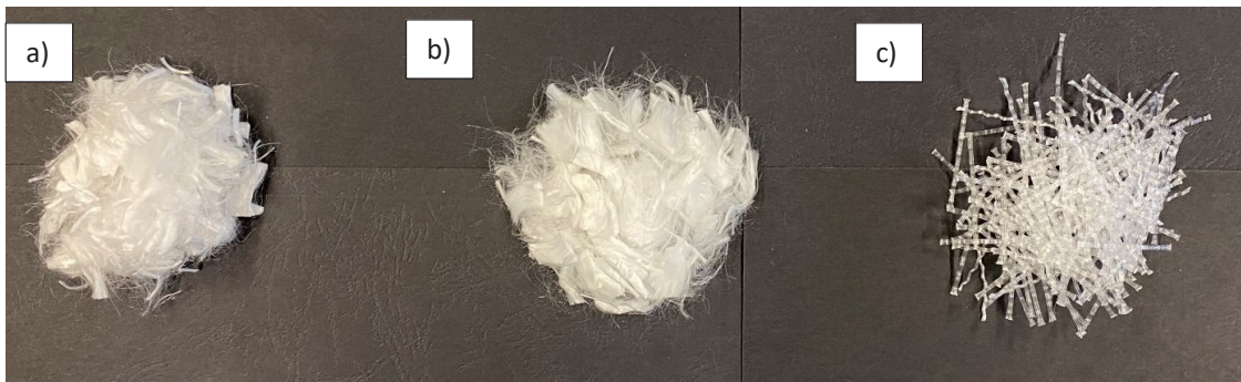
Figure 2: Different lengths (and diameters) of fibres in the amount of 0.2% in reference to the dry mass of the sample that was added to the coarse soil: a) 12 mm (0.030 mm), b) 18 mm (0.034 mm), c) 40 mm (0,90 mm).
