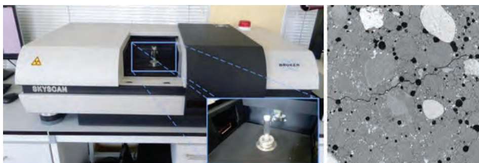
Fig.19. A stand for an x-ray examination with computer microtomography and an example of a concrete cross-section, according to [42]
