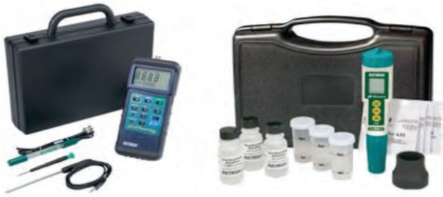
Fig. 17. View of the newest set to assess the pH of concrete [36]
