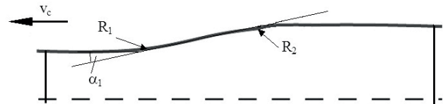
Fig. 7. An outer profile of the bimetallic tube during the simultaneous pre-drawing with marked output radius R_1 , the output angle \alpha_1 and input radius R_2
