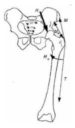
Fig. 2. The active model of loads in the hip joint [1]
