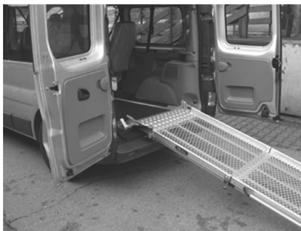
Figure 5 FEAL overrun platform, assembled by Cebzon
