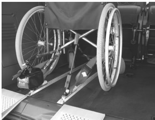
Figure 6 UNWIN overrun platform, assembled by Cebzon
