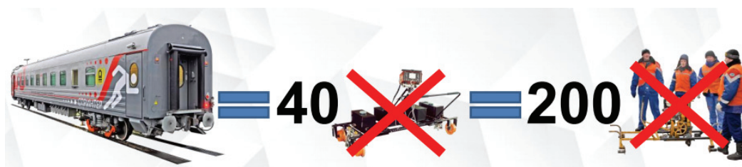
Fig. 15. One flaw detector car eliminates 40 manually operated devices and 200 people necessary to operate them [11]
