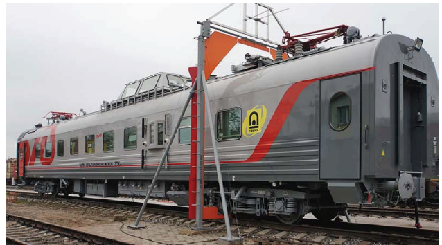
Fig. 5. The Integral car on the measuring instrument calibration station [19]
