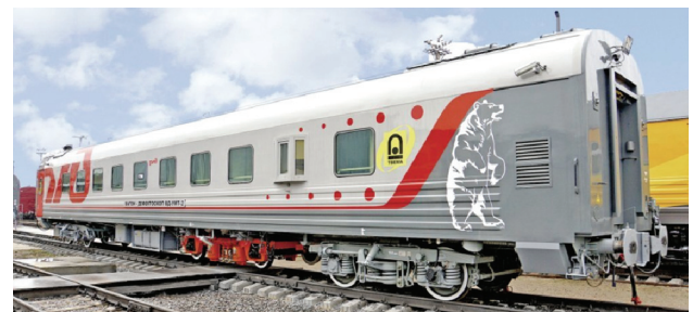
Fig. 6. The VD-UMT-2 flaw detector car is designed for complex diagnostics of railway infrastructure using ultrasonic, magnetic and optical non-destructive testing methods [17]
