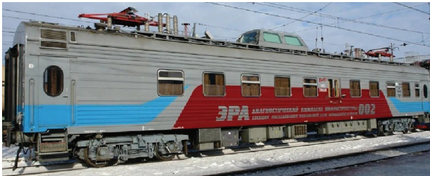
Fig. 4. Testing car for overhead contact line, ERA automation and remote-control devices [14]
