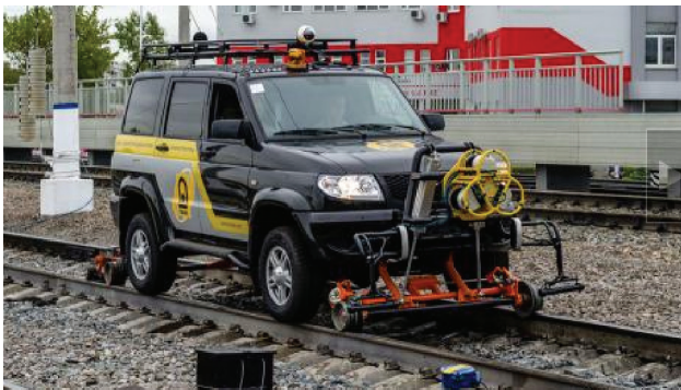
Fig. 14. Road vehicle used for trackside infrastructure measurements [12]
