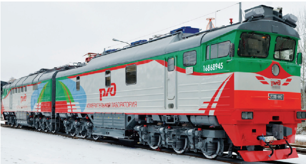
Fig. 10. SMDL- 2TE116 measuring diesel locomotive [6]; a) View of the locomotive, b) Rail condition laser monitoring devices, c) GPR for monitoring the substructure, d) Overhead contact line condition monitoring equipment
