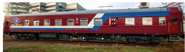
Fig. 3. RDM – WIGOR flaw detector car [14]
