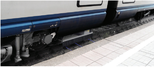
Fig. 12. Sapsan train laser device for rail condition measurement [5]
