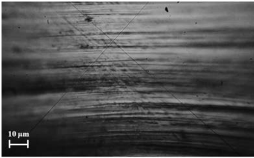
Fig. 2a. Optical image of the surface of an example block before the wear tests
