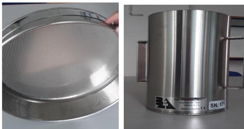
Figure 3. A 5 l stainless steel cylinder and a round sieve with 3.15 mm mesh diameter, 400 x 100 mm
