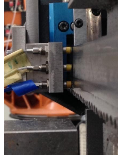
Fig. 5. Measurement principle with three eddy current sensors for the displacement of the saw blade
