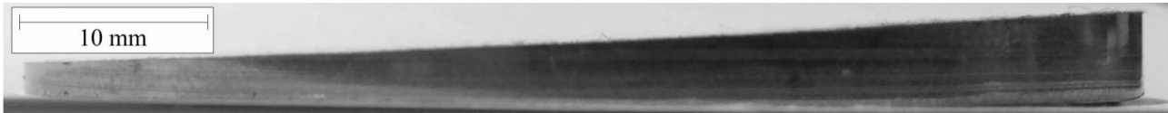
Fig. 10. Side view of a workpiece with a great cutting deviation (steel grade: 42CrMo4)
