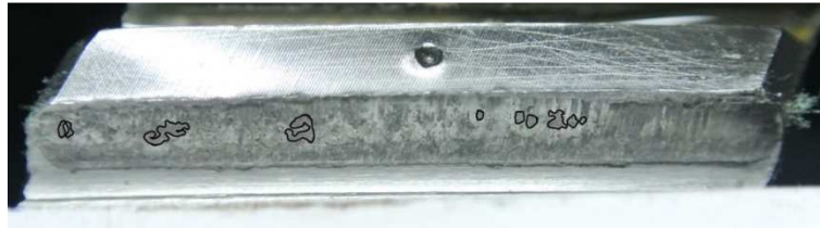
Fig. 20. Pitting on wheel tooth of tested Novikov gear after fourth load stage
