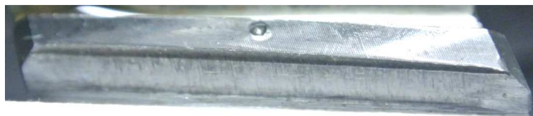
Fig. 15. Pinion tooth surface of tested Novikov gear after second load stage
