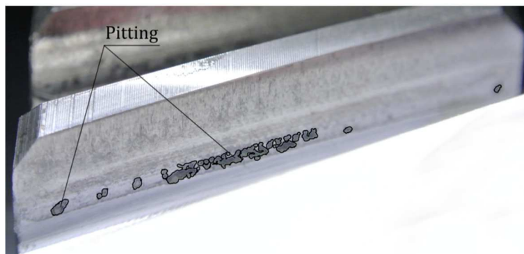
Fig. 8. Pitting on pinion of tested involute gear after third load stage
