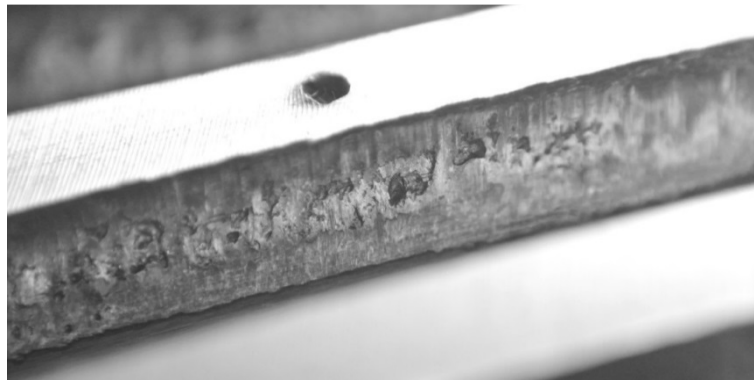
Fig. 27. Macrograph of pitting on pinion tooth surface of Novikov gear
