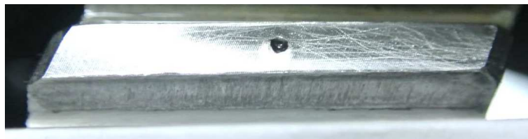
Fig. 18. Wheel tooth surface of tested Novikov gear after third load stage
