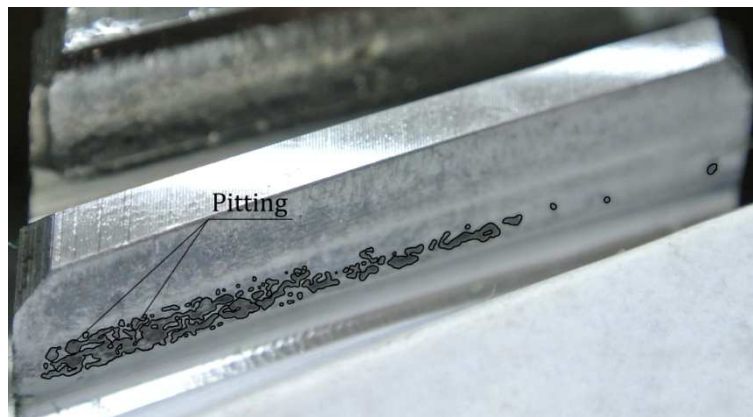
Fig. 12. Pitting on pinion of tested involute gear after fifth load stage
