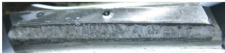
Fig. 21. Pitting on pinion tooth of tested Novikov gear after fifth load stage
