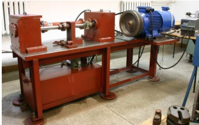
Fig. 1. Closed loop power circulation test stand, based on [21]
