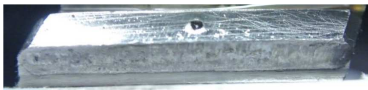
Fig. 22. Pitting on wheel tooth of tested Novikov gear after fourth load stage
