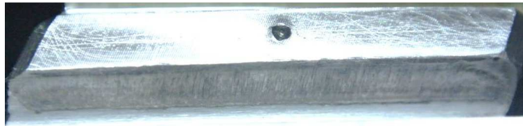
Fig. 16. Wheel tooth surface of tested Novikov gear after second load stage
