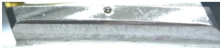
Fig. 17. Pinion tooth surface of tested Novikov gear after third load stage
