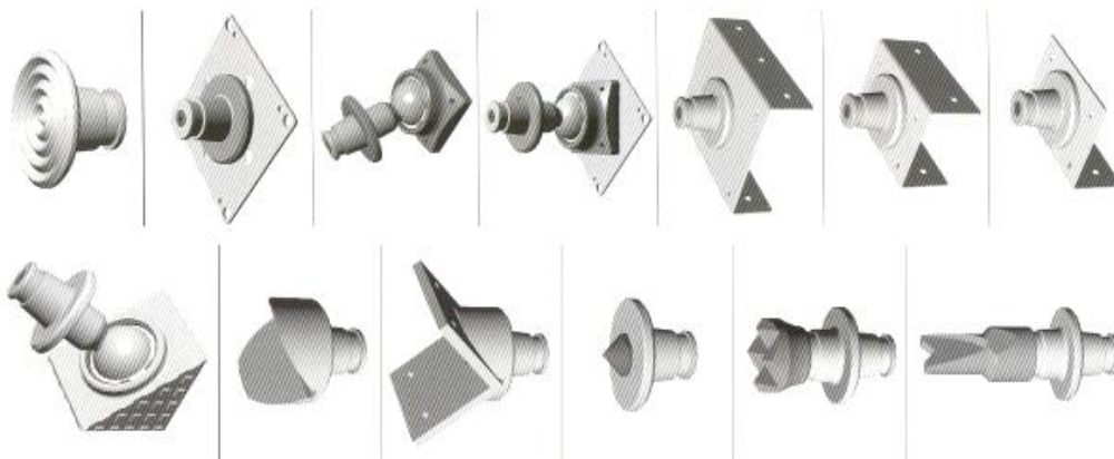
Fig. 6. Exemplary shapes of working tips of spreading cylinders
