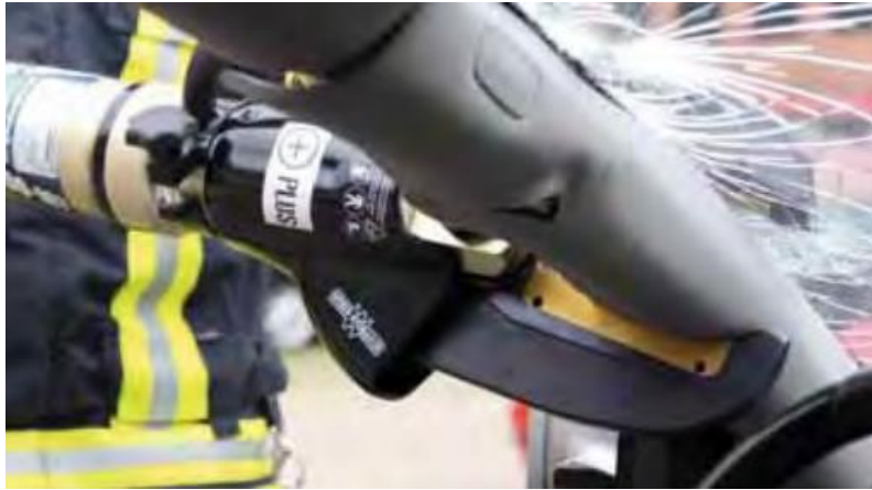
Fig. 5. Example of using a hydraulic cutter to cut an A door pillar in a vehicle
