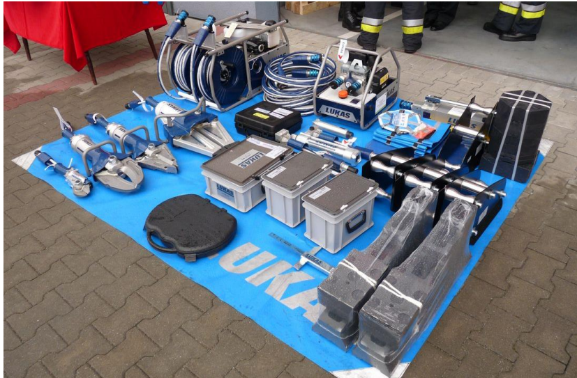
Fig. 1. Exemplary hydraulic rescue kit manufactured by the Lukas company
