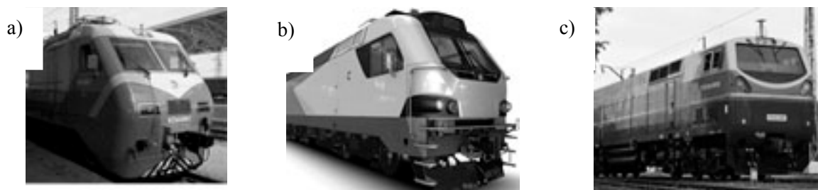
Fig. 1. The new locomotives operated on the railroad of the Republic of Kazakhstan: KZ4AC (a), KZ8A (b), TE33A (c)
