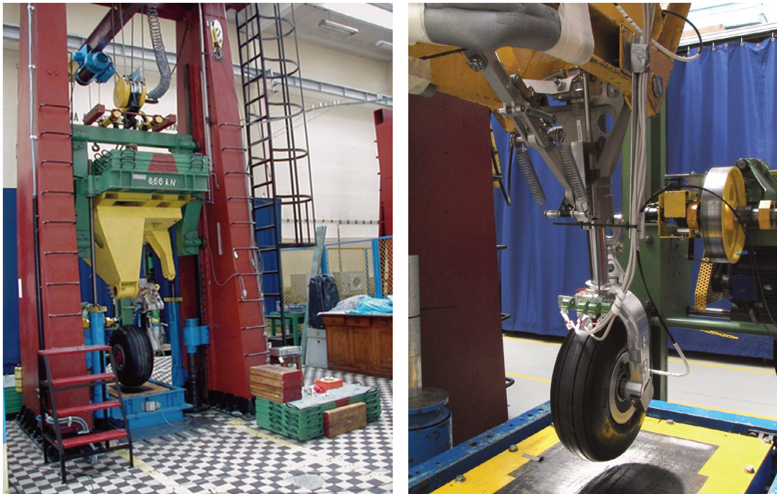
Figure 7. M10T test stand – overview example (left), I-31 NLG mounted (right).
