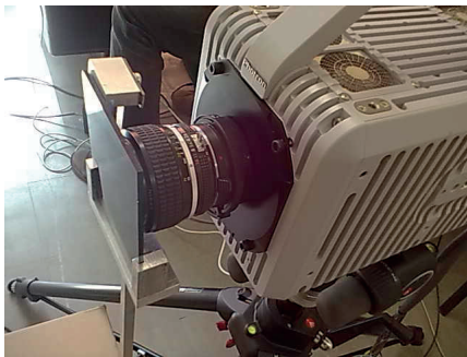
Fig. 5. View of the high-speed camera and the light-blocking filter used during the tests
