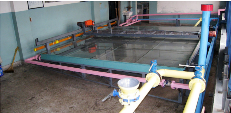
Fig. 1. Model body of simulation ventilation network
