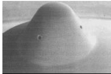
Fig. 2. Fuel injection nozzle cap holes machined by FS laser [41]
