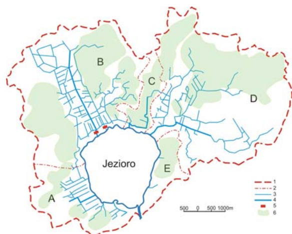
Fig. 1. Hydrographic Network within the catchment of the lake (Jezioro); 1 = border of the catchment; 2 = borders of sub-catchments; 3 = ditches with width below 5.0 m; 4 = channels (ditches) with width over 5.0 m; 5 = pump station; 6 = drainage infrastructure; source: own elaboration
