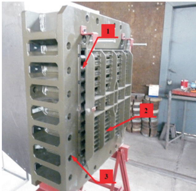
Fig. 1.2. Main components of a explosion-proof valve: 1 — stopper grate, 2 — moving grate, 3 — body
