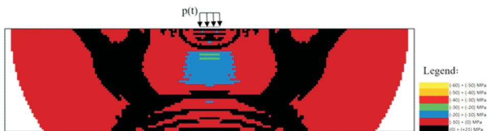
Fig. 3.3. Distribution of normal stresses acting in the direction of the load p(t) in the analysed shield at 117.80 \mu\text{s}
