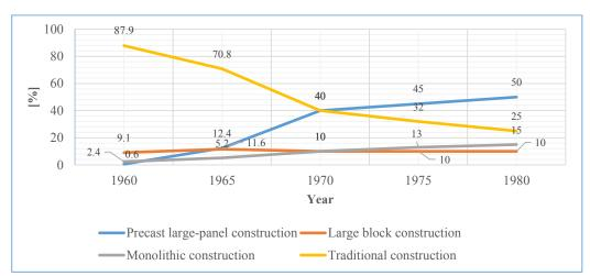
Figure 1 Summary of rooms planned to be constructed with a breakdown into individual construction methods in the 1960-1980 period [2, 3]
