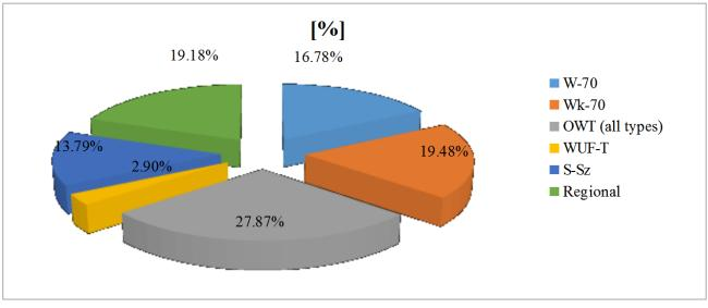
Figure 2 Graph showing the percentage share of individual precast large-panel systems in Poland in the 1970-1985 period [3, 8]
