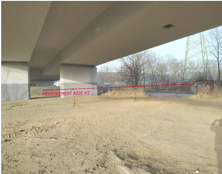
Fig 15. Axis #2 was placed on unpaved ground (below the slope). Source: author's Piotr Kozłowski own photo archive
