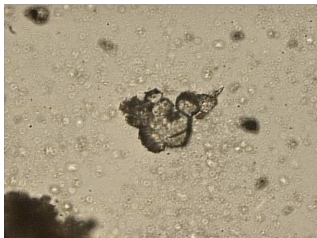
Fig. 1. Idiomorphic olivine crystals with characteristic high relief, one nicol, magnification 400x.
