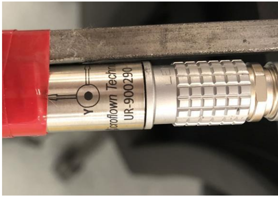
Fig. 5. Microflown USP sound intensity probe
