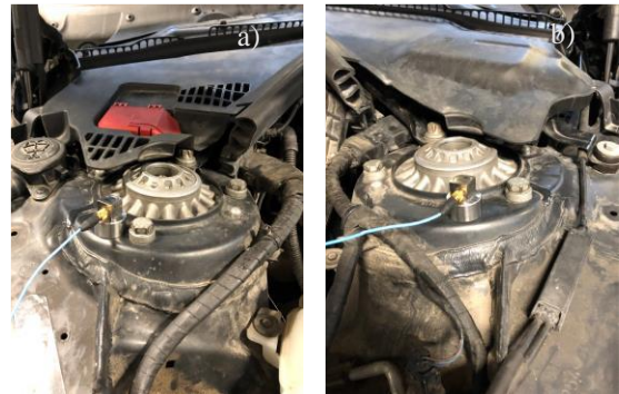
Fig. 3. Excitation sites – BMW a) right tower passenger b) left tower driver
