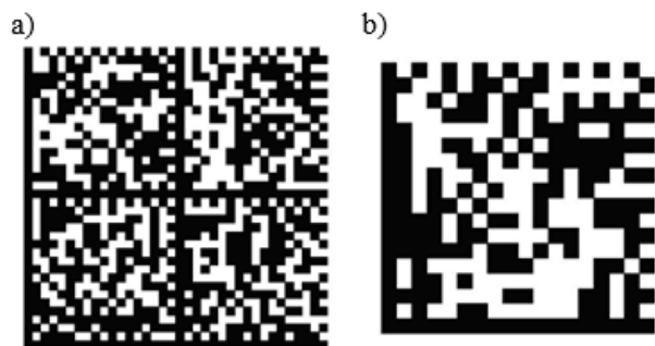
Fig. 1. a) DataMatrix symbol encoding the following text: a) "This is a very long text encoded in DataMatrix. In order to ensure easier decoding, the symbol has been divided into sections"; b) A DataMatrix symbol encoding a short text (Langman et al., 2007).
