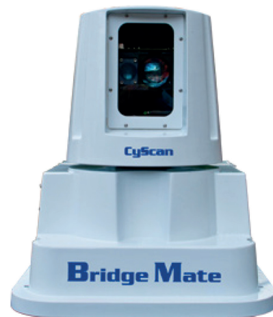
Fig. 5. Cyscan laser sensor with revolving head [4]
