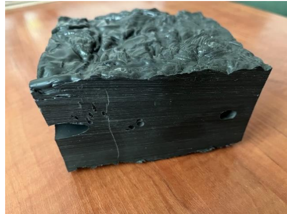
Fig. 4. Example of poor structure of an HDPE product cast without regime pressure
