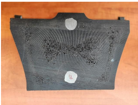
Fig. 3. Cross-section of the investigated sleeper – middle part of the sleeper
