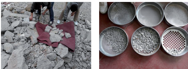
Fig. 1. Selection and screening of waste road concrete
