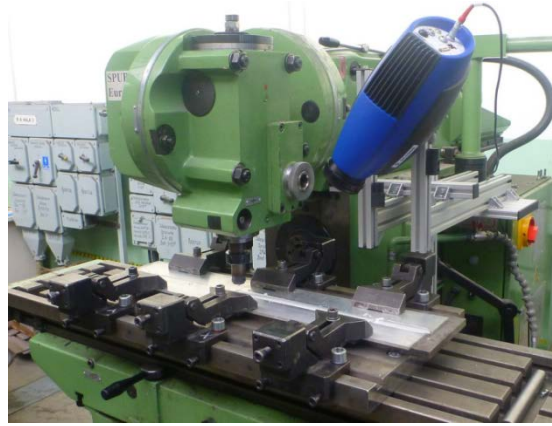
Fig. 3. The view of the research stand for monitoring the FSW process with installed thermal imaging camera
