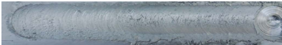
Fig. 10. The view of the weld surface
