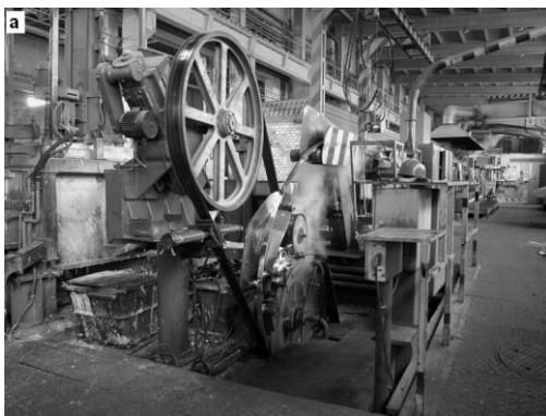
Fig. 1. View of the casting line: a) Continuous Casting and Rolling: Continuous Properzi, b) Laboratory line of continuous casting
