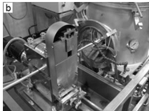
Fig. 1. View of the casting line: a) Continuous Casting and Rolling: Continuous Properzi, b) Laboratory line of continuous casting
