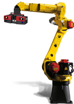
Fig. 2. Industrial robot with optical measuring system GOM Atos Triple Scan
