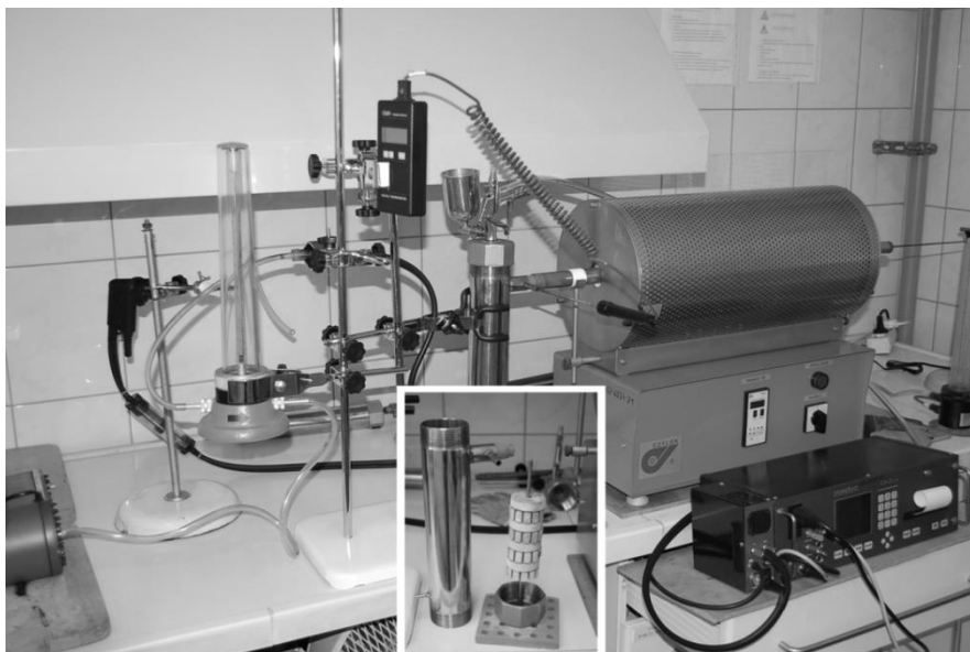
Photo 1. Installation for experimental studies on the removal of \text{NO}_x using SCR method; in the middle baffles with catalyst
