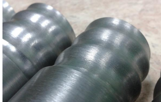
Figure 2. Example of a rope thread in one-pass threading
