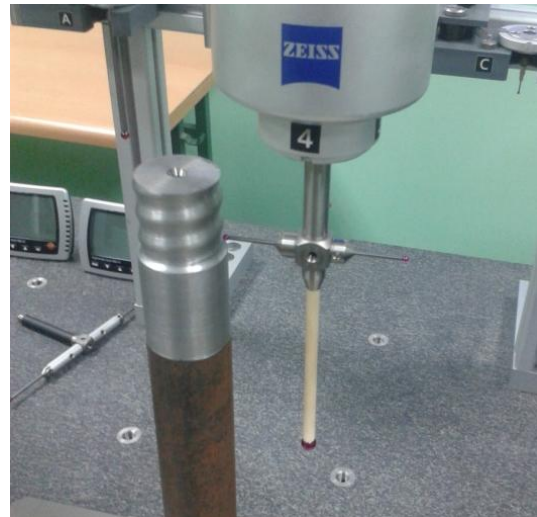
Figure 8. View of a rope thread sample during geometry measurements performed with CMM
