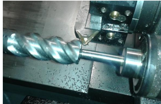
Figure 1. Example of a trapezoidal thread in one-pass threading
