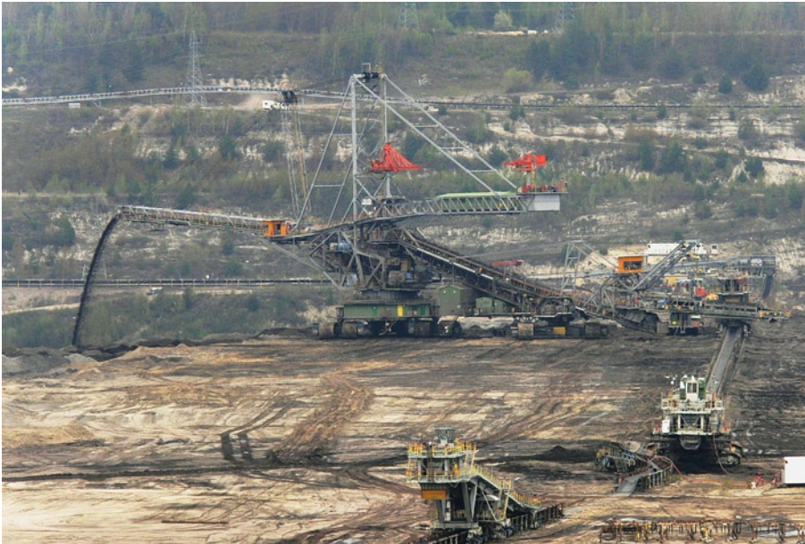
Fig. 1. Spreader A 2 RsB 15400 – typical example of opencast mining machinery (photo. P. Grabowski)
