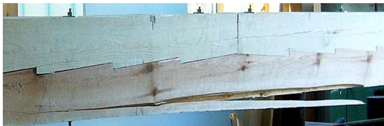
Fig. 11. Specimen 01 – tensile fracture on the bottom surface
