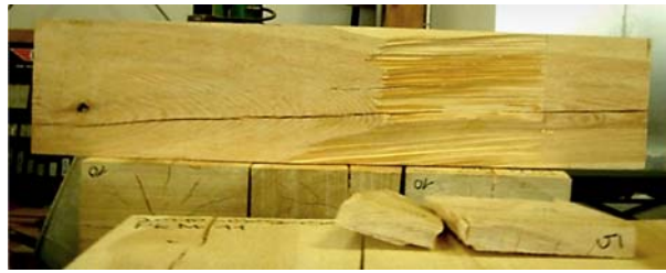
Fig. 8. Shear fraction on a tooth joint – specimen No. 5 (scale 1:1)
