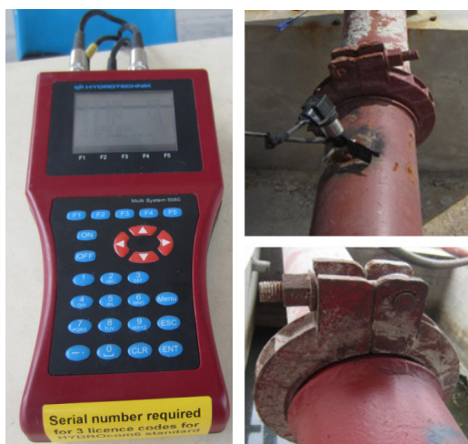
Fig. 3. MultiSystem 5060 portable tester
