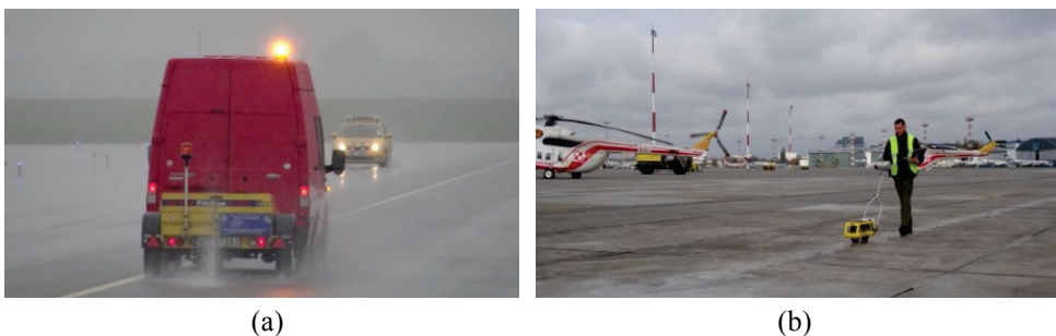
Fig. 2. Airport surface friction tester (ADFT) on T-10 trailer (a); manual, portable, air port surface friction measuring equipment T2Go (b) [source: archive of AFIT]
