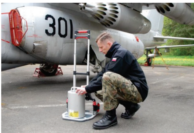
Fig. 4. Device ELATextur for the measurement of macrotexture [source: archive of AFIT]
