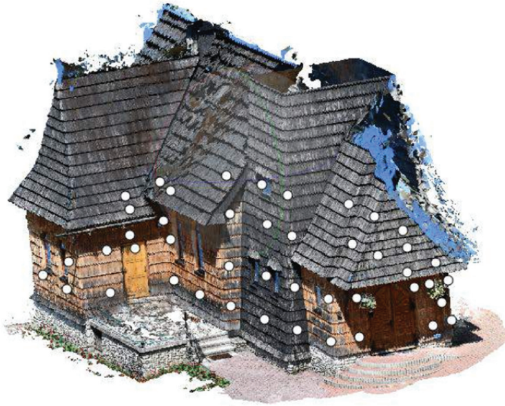
Fig. 6. Dense point cloud (Nikon D7500 non-metric camera)
