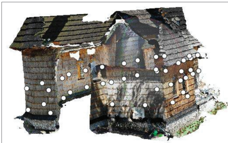
Fig. 9. Model of the south-western wall obtained using the UAV
