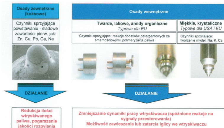
Fig. 2. Types of deposits formed inside and outside of the injectors in HPCR injection systems, factors facilitating their formation and impact on engine operation
